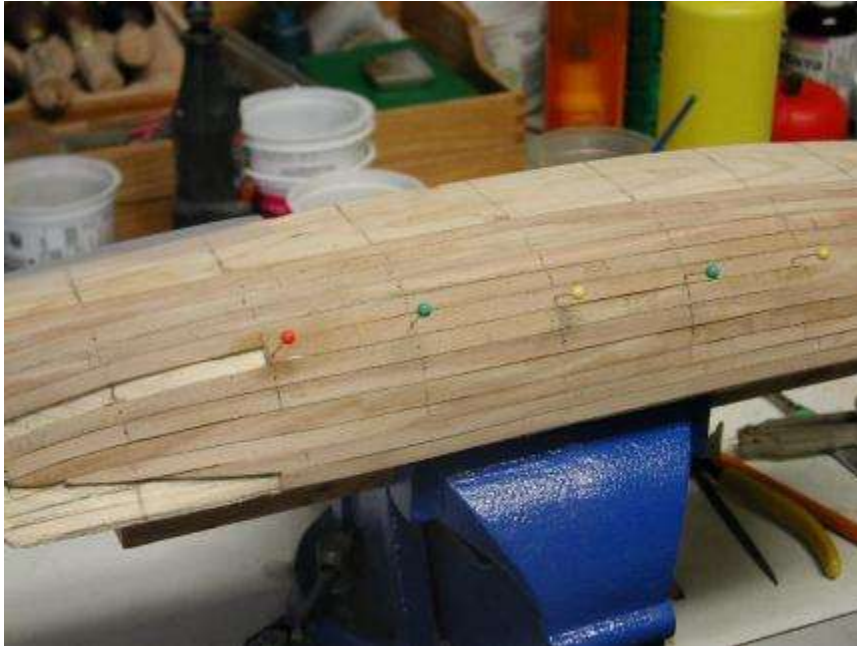
Above. Midship plank installed.
