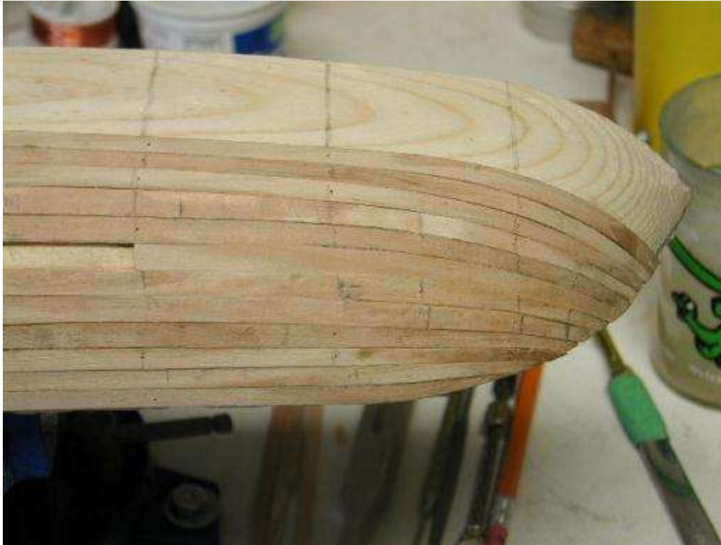
Above. First plank at stem installed.
